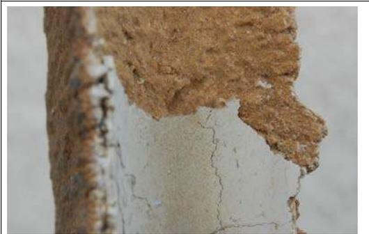
**Figure 6.** High Deposit on superheater tube. Note the first white layer composed of sub micron particles and alkali vapor condensation.
